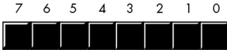
Figure 2-3: Bit numbering in a byte
