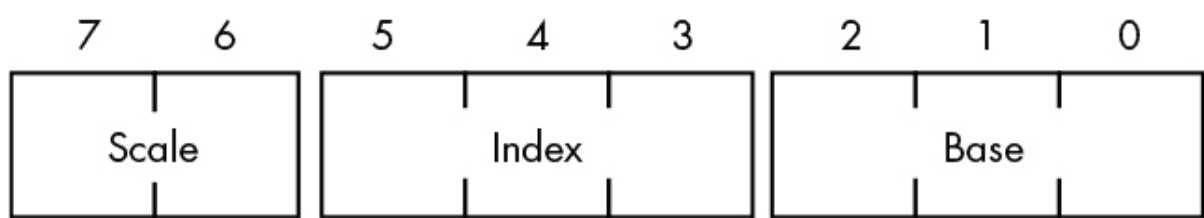
Figure 10-17: The sib (scaled-index byte) layout
