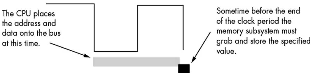
Figure 6-18: A typical memory write cycle
