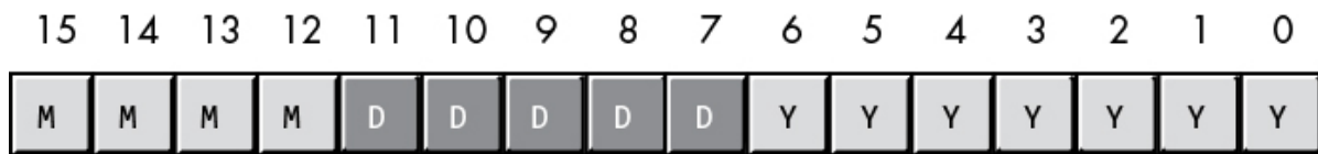
Figure 3-6: Short packed date format (16 bits)
